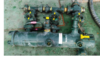
Cement Head Assembly
