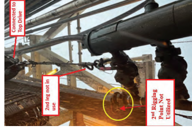
Original Sling Configuration to Cement Head D-Link Only (1 x Attachment Point and One Leg used)
