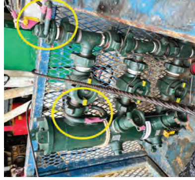
Cement Head configuration can accept a 2nd slinging point to allow better vertical orientation & reduce risk.
