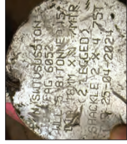
2 Leg Sling Tag recovered post incident.
