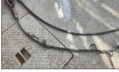
2-Leg Slings Single Leg Damage
