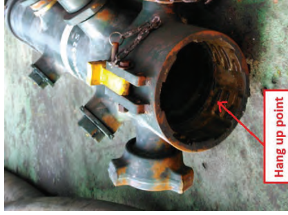
Cement Head Quick Release Latch Close-up
